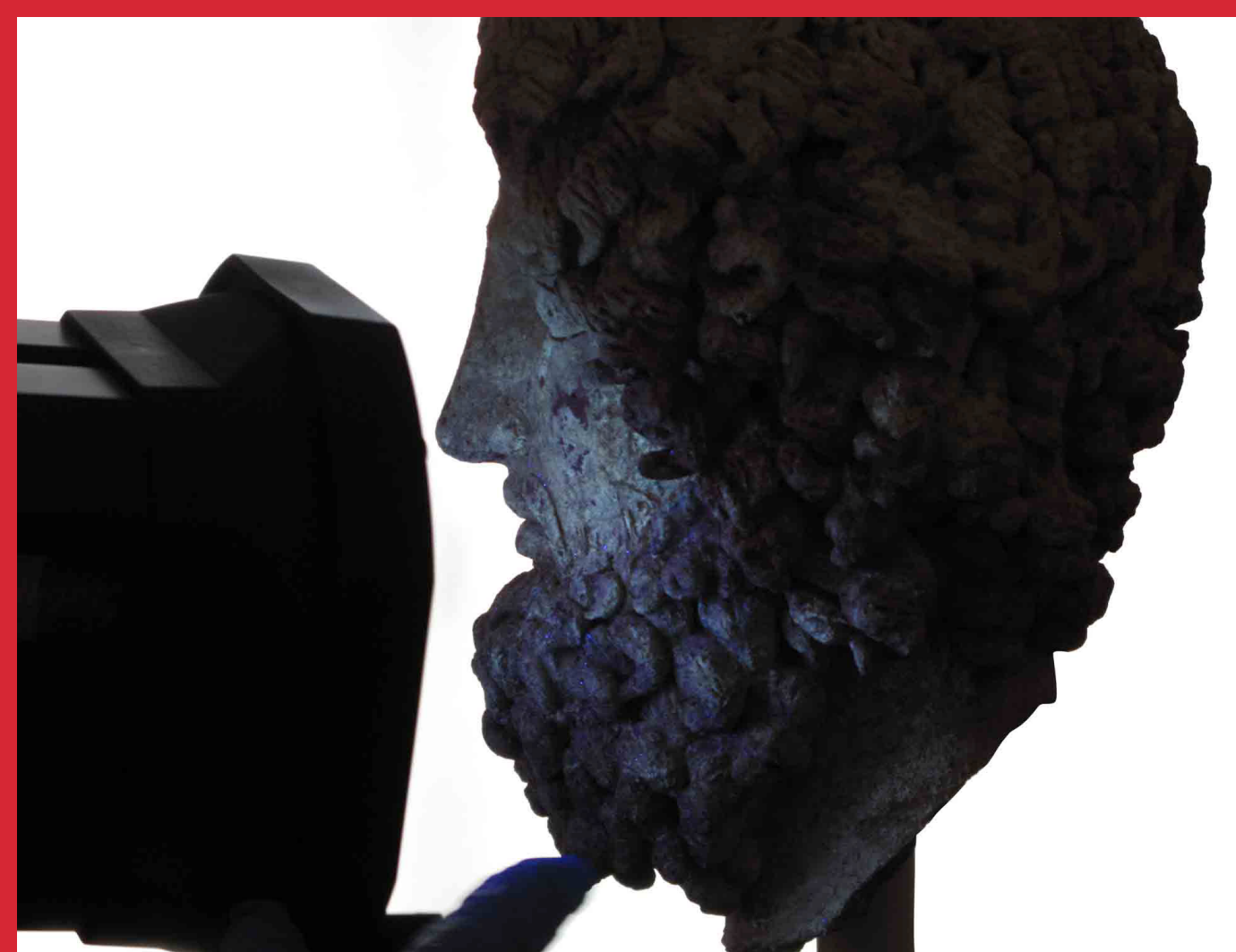
Figure 2 - UV observation of the face that shows yellowish and blue-violet fluorescence.
