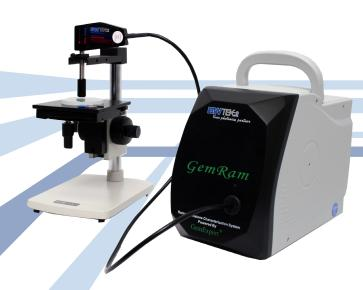
The GemRam is a lightweight, portable Raman spectrometer dedicated to both the verification of known gemstones as well as the identification of unknown gemstones. It comes equipped with B&W Tek's GemID identification software, powered by GemExpert's spectral library of nearly 300 different gemstones, as well as unlimited space for user defined spectra that can be added at any time.
